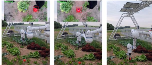
Fig. 7: Validating the simulated algorithm with plastic balls
